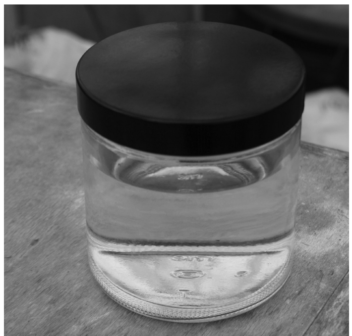
Figure 1. A jar test can be used to determine physical compatibility of pesticides.
