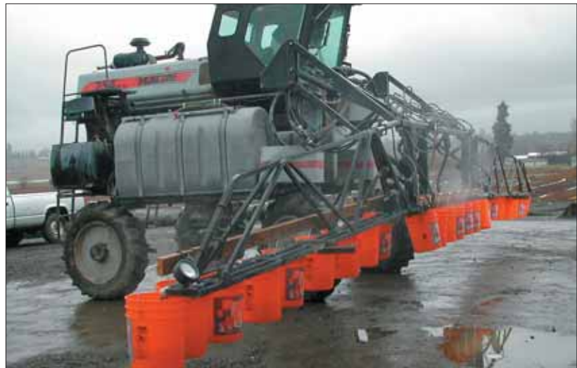
Figure 10. Buckets hang from this boom sprayer to verify that output is uniform between nozzles.
