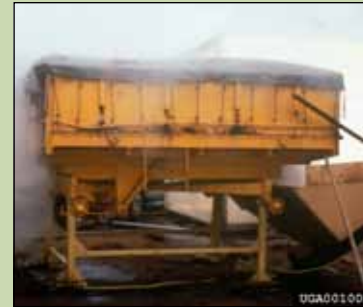
Fig. 7.2.1.d. — Aerated steam treatment of containers in a free-standing loader. Photo courtesy of T. Landis, USFS, www.bugwood.org .
