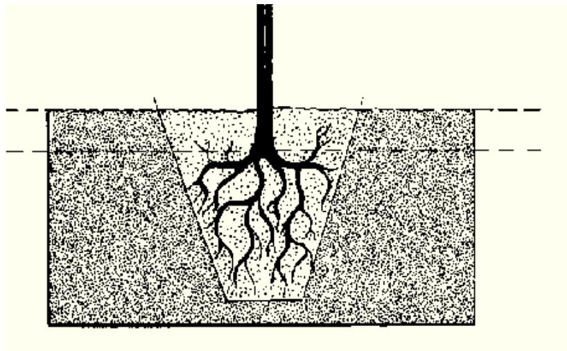
**Figure 8. Cultivating can cause soil buildup high around the collar of nursery stock, creating a false soil line, as illustrated above. Planting at that false line is harmful to the health of the tree.**
