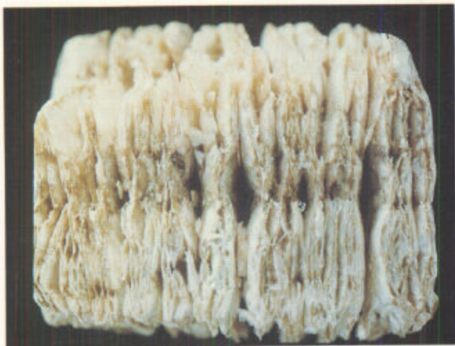
Figure 2.2.11 —Horticultural vermiculite particles (A) are accordion-like, because of their expanded structure of parallel plates (B), which creates an extensive internal surface area (B, courtesy of Biamonte 1982).
