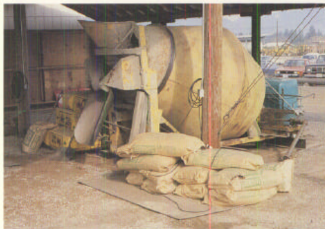
Figure 2.2.18 —Various types of equipment have been modified for custom-mixing growing media, including small portable cement mixers (A) and converted concrete trucks (B).
