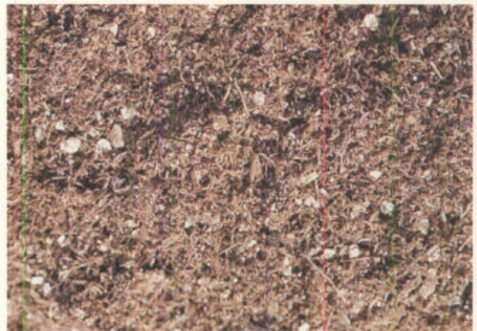
Figure 2.2.21 —A well-mixed growing medium should have a uniform composition with minimal damage to the size or shape of the original components, in this case sphagnum peat moss and vermiculite.
