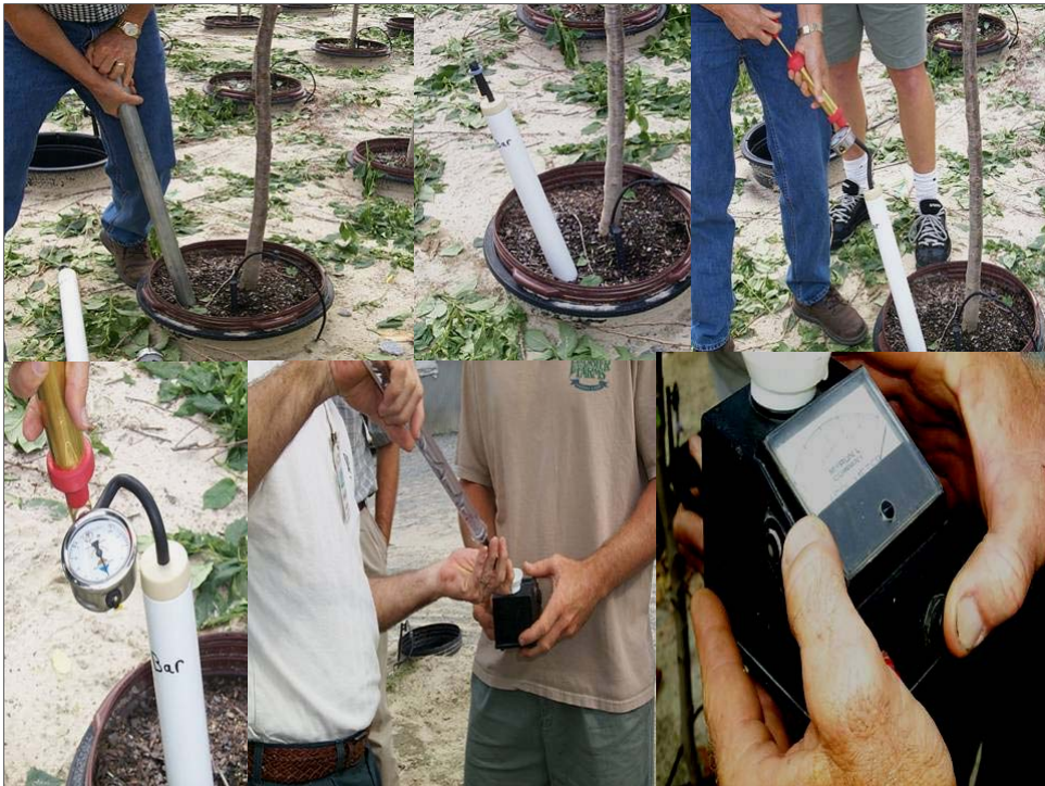
The composite of slides shows steps for installation and extraction of solution from lysimeters. The vacuum pump is seen in the upper right and lower left picture.
