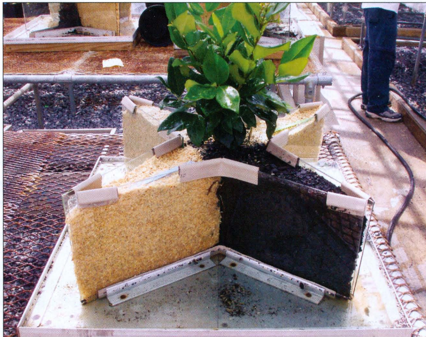
The Horhizotron is used to evaluate root growth of woody shrubs in PTS and pine bark.
