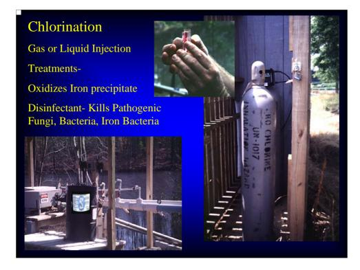
A swimming pool test kit is used to colormetrically determine free chlorine concentrations in irrigation water. Any coloration shown at the end of the irrigation line indicates the presence of free chlorine and therefore indicates that disinfection has been effective. Concentrations of 0.5 pp to 2.0 ppm free chlorine are considered acceptable.
