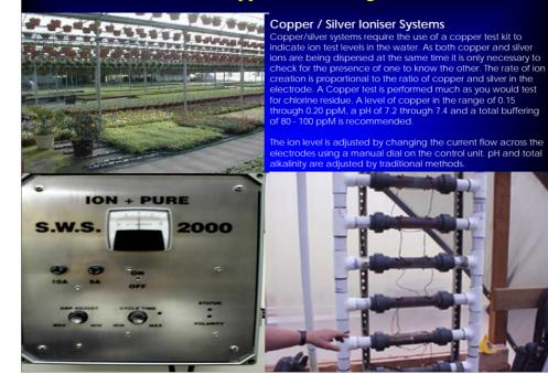
Copper/Silver ion generators are occasionally used at nurseries. The free Cu ion concentration must be kept below 2.0 ppm or root inhibition will occur in nursery crops. Most Cu/Silver ion generators maintain Cu concentrations below 1.0 ppm.
