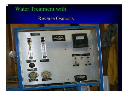
Reverse Osmosis may be one of the most expensive systems per gallon of treated water. Most RO systems have limits of water treatment such as less than 100 gallons per day. I have seen only one RO system in use at a Texas nursery with high NaCl concentrations in water supplies. The RO system was being used to purify water for a propagation greenhouse range.
