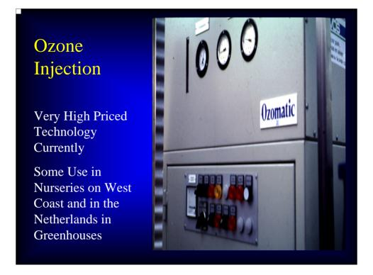
Ozone injection is also an infrequent technology used for treatment of nursery irrigation water supples. The unit pictured above was seen in a very advanced greenhouse facility in the Netherlands. Ozone was also being used at a nursery visited in Oregon for disinfection of irrigation water used for propagation greenhouses. An Ozone test kit, much like a test kit used for testing chlorine in swimming pool water is used to determine appropriate concentrations.
