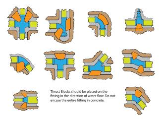
Figure 2. Thrust block (orange in figure) placement.
