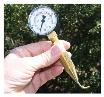
Figure 4. Pitot tube for measuring dynamic or working water pressure at the nozzle. (Photo courtesy of David Ross, Univesity of Maryland.)
