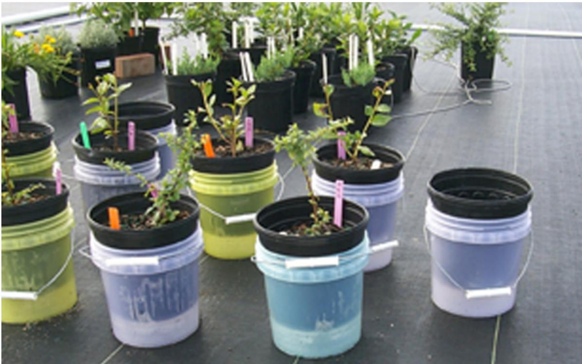
Irrigation water volume collected buckets under plant containers represent the leaching fraction volume during an irrigation cycle. Water volume collected in empty containers represents the total water volume applied. To determine leaching fraction (LF) divide the
