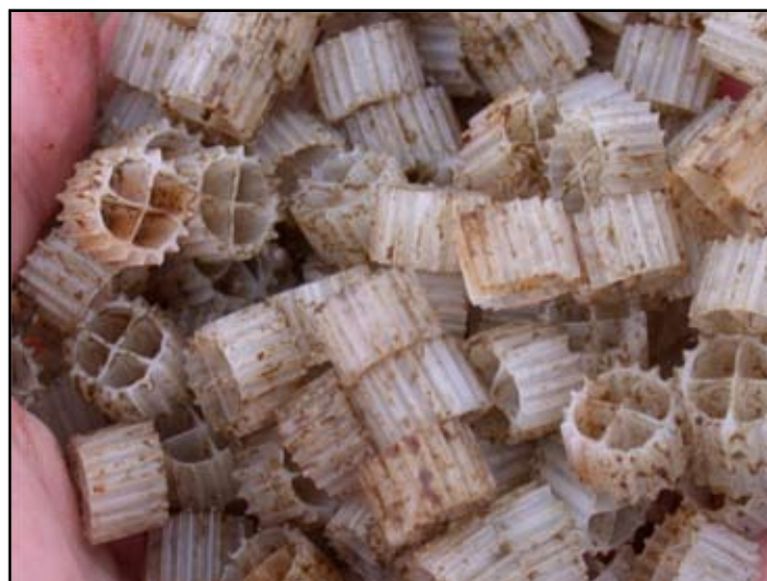
Figure 1. Kaldness media inoculated with denitrifying microorganisms.
